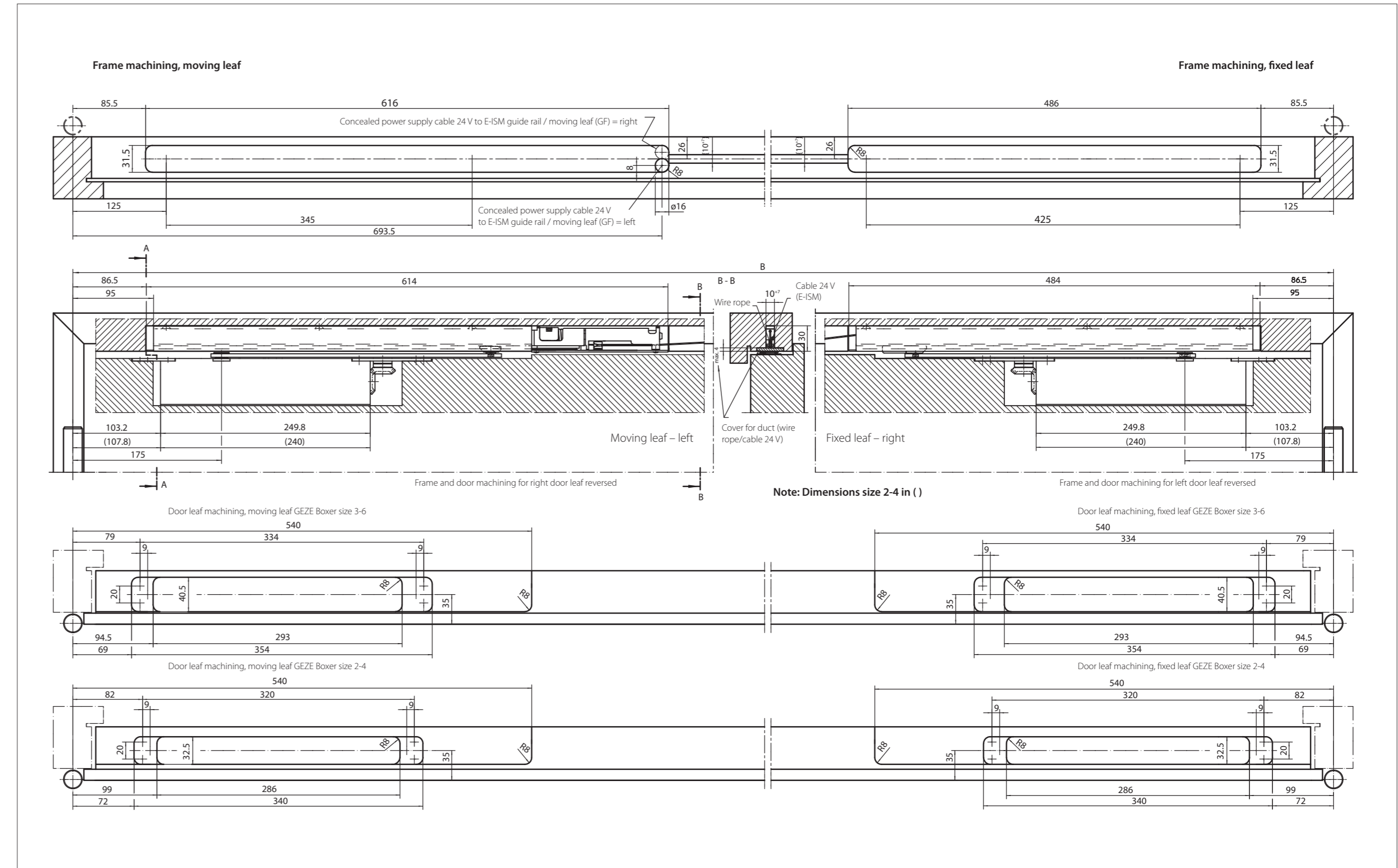
Fig. 13-1 · ISM/E-ISM guide rail Boxer size 2-4/3-6, rebated timber door
