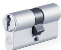
Cylinder with janitor function No. 810/59 Master key operates bolt and latch. Single key operates the latch only. For hotel interconnect- ing doors, schools etc.
