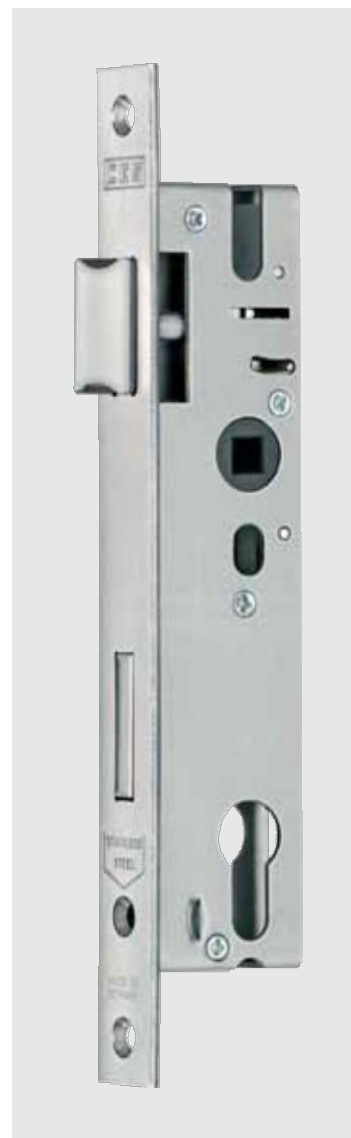
CES mortise lock 5834 medium version 20, 25, 30, 35, 40, 45 mm backset forend 24 x 245 mm edged with transmission bar prepared for profile cylinders only one turn bolt space 15 mm
