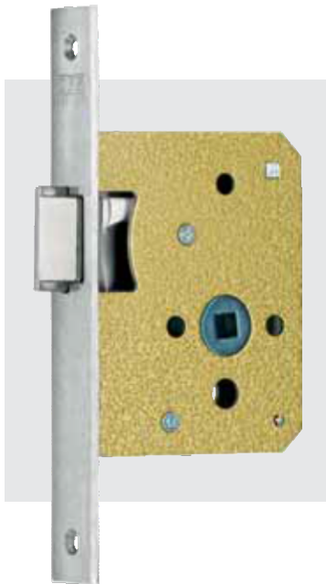
CES mortise lock 2500 only latch bolt 55, 60 or 65 mm backset forend 24 x 185 mm, edged or rounded not reversible (left or right hand)
