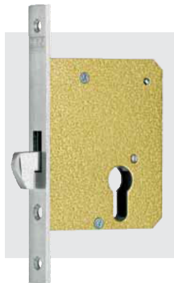
CES mortise lock 5830 for sliding doors only 55 mm backset forend 20 x 168 mm, edged
