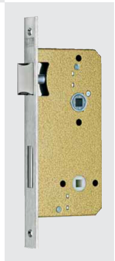
CES mortise lock 9090 85 mm distance 8/8 mm follower bathroom lock
