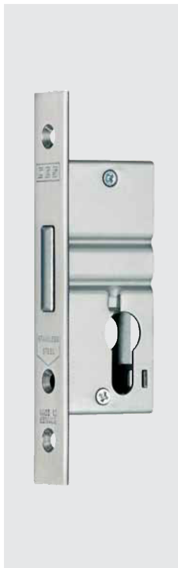
CES mortise lock 5530 25, 30, 35, 40, 45 mm backset forend 24 x 160 mm edged prepared for profile cylinders only dead bolt
