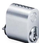
Scandinavian cylinder No. 5746 outside version basic length: 25,7 mm 5 and 6 pin system
