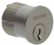
3902 Mortise Cylinder • Conventional cylinder supplied drilled 6-pin, keyed 5-pin standard • 3975 standard cam attached and 3972 Adams Rite cam shipped loose in the box • Thread size is 1.150" x 32 UNS • Cylinder face diameter is 1.360" • Supplied with two operating keys • 1-1/8" (29 mm) standard length, 1-1/4" (31 mm), and 1-5/8" (41 mm) for mortise exit devices • Other lengths may be available with extended lead time • Must specify length, cam, keyway, and keying requirements
