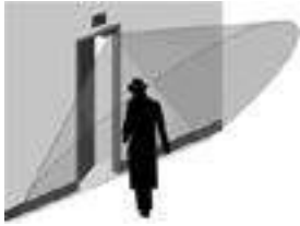
Embedded CCTV captures full facial view of persons exiting door
