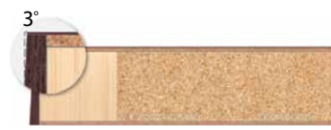
Lipped two edges in Ash and edge banded to match face
