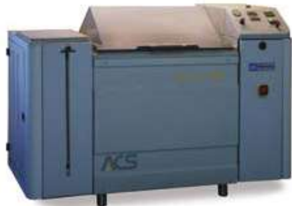
Salt spray chamber: Angelantoni ACS mod. DCTC600.
